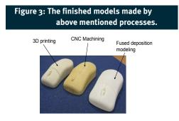
off between cost and quality arises. For large models, as surface finishing is a minor concern, CNC machining is appropriate because it is cheaper and less time consuming while, for small and precise models with intricate shapes, fused deposition modelling is the best option because for small scale models surface quality is more important than cost.
